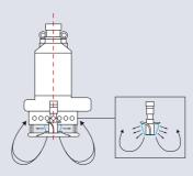
The rigid agitator delivers kinetic energy (energy of motion) to stir solids surrounding the pump intake, re-suspending them into a fluid state for easy pumping.
